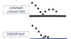
An undamped urethane returns nearly all of the impact energy, while Confor® foam absorbs it.
